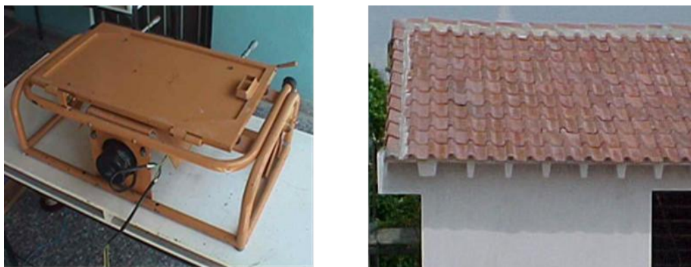
Fig. 1-TEVI technology. a) TEVI roof tile production machine. b) TEVI tile roofing.
