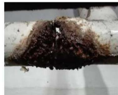
**Figure 12.** Break in pipes
